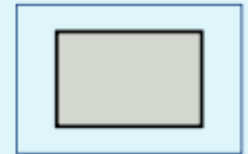
APS-C (Nikon DX, Pentax, Sony) \sim 23.6 \times 15.7 \text{ mm} \sim 370 \text{ mm}^2
