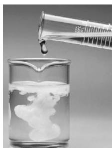
The precipitation reaction that occurs when yellow potassium chromate, K_2CrO_{4(aq)} , is mixed with a colorless barium nitrate solution, Ba(NO_3)_{2(aq)} .
