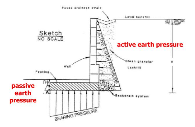
Granular soils (sands or gravels) are the standard recommendation for backfill material.
