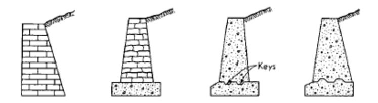
Gravity retaining walls are routinely built of plain concrete or stone, and the wall depends primarily on its massive weight to resist failure from overturning and sliding.
