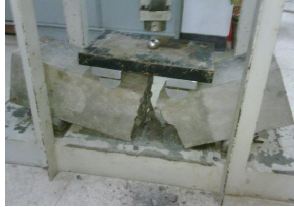
Fig. 2. Third point loading test for concrete beam specimens [10]
